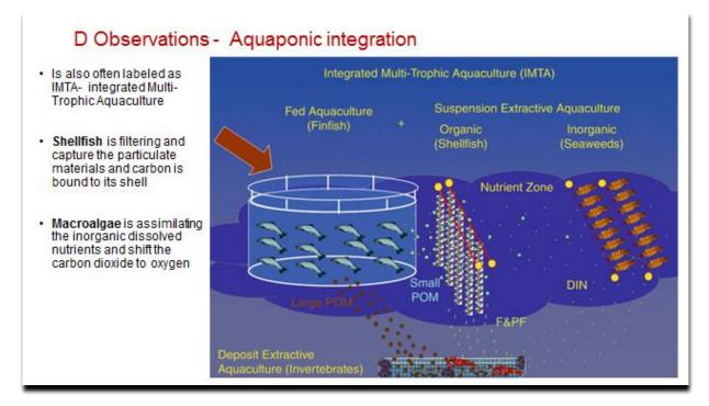
Figure 5. Illustrations of aquaponic setup.
