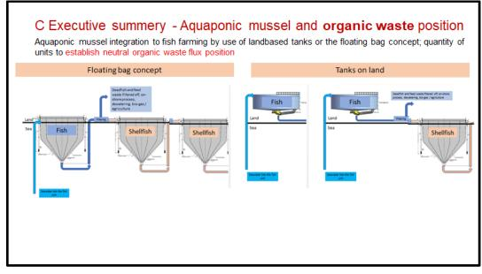
Figure 61. Integration of mussel aquaponic unit to on land and offshore fish farms.
